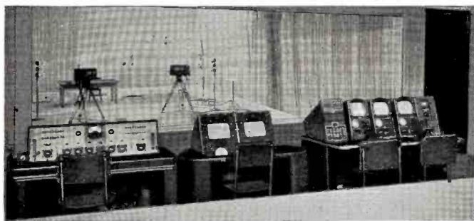
Control and studio equipment at KSD-TV includes (left to right) a control console, master film and camera monitors, a switching unit, three camera controls, a sync. generator and, back-ground, two image-orthicon cameras.
